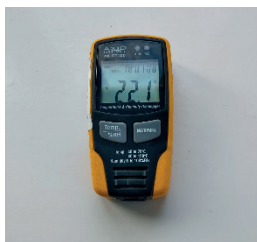
Figure 3. AX-DT100 logger for temperature and humidity measurements
