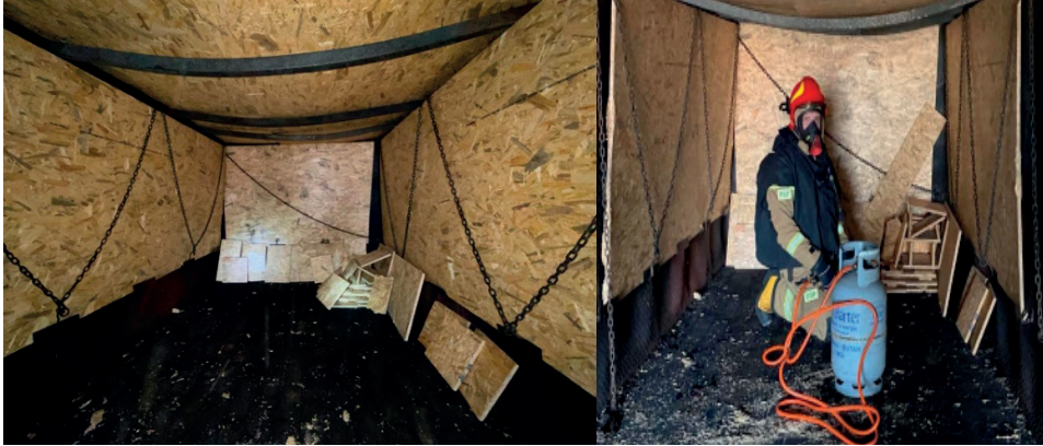
Figure 4. Fire chamber prepared for fire tests
